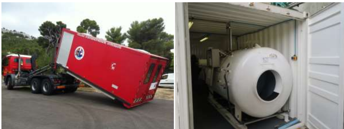
Figure 13 : Caisson de recompression mobile (Source : Mathieu Coulange)
