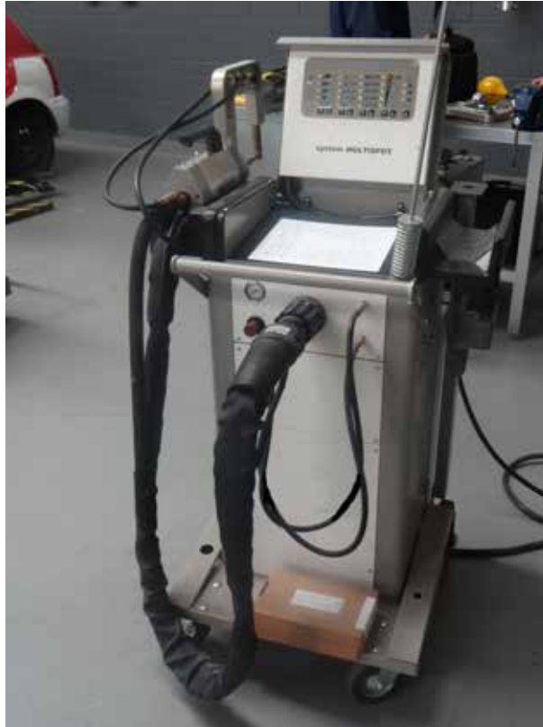
Figure 6.2 — A typical body repair shop hand-held spot welder. The system is mobile with the control unit on castors. Electrical and coolant supply cables leave the front of the unit and feed into the rear of the welding gun, which is sitting in its holder to left of the control panel
