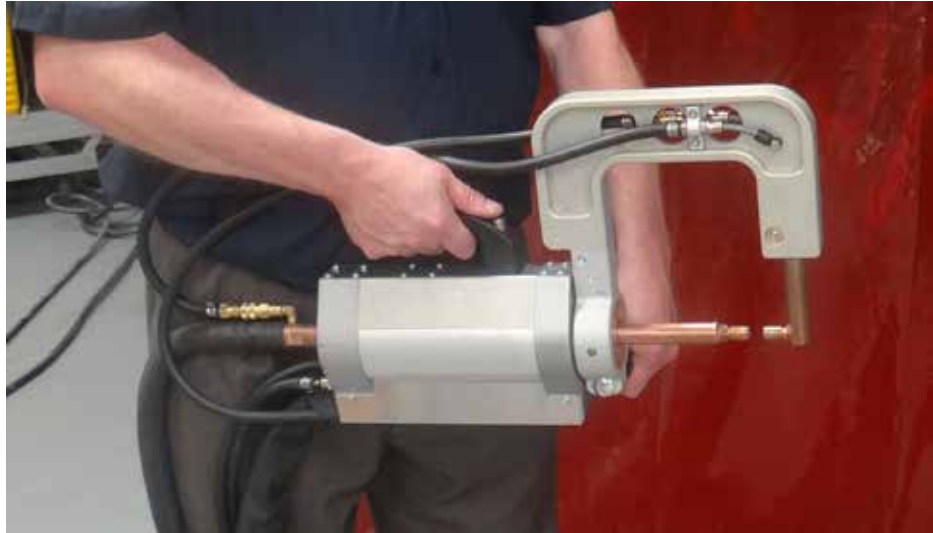
Figure 6.4 — The repair shop ‘C-type’ welding gun, with the 160 mm arm fitted. The main body of the gun (under the worker’s hand) contains the piston that forces one electrode onto the other. The welding current is delivered from the control unit by the cables to the left of the picture
