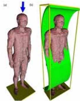
Figure D11 — Example 1: Human model exposed to an electromagnetic field reflected back into region occupied by the human. This region is shown as a yellow box. The standing wave is shown in green.
